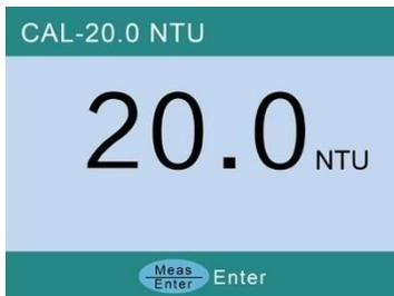
7) After calibration with 20.0 NTU standard, press key to return to calibration menu.
