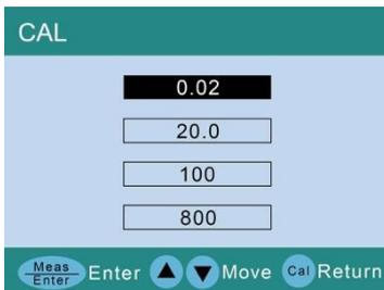
4) Press key to enter calibration menu, and press key to perform calibration when cursor is on 0.02.
