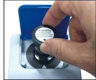
3) Open the flip cover and put in 0.02 NTU calibration vial. Align the arrow on the vial with the arrow on the sample well and then close the cover.
