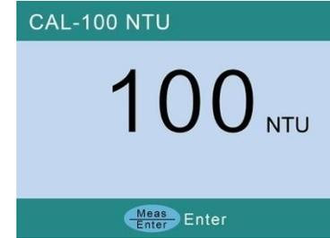
9) After calibration with 100 NTU standard, press key to return to calibration menu.
