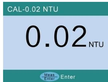
5) After calibration with 0.02 NTU standard, press key to return to calibration menu.
