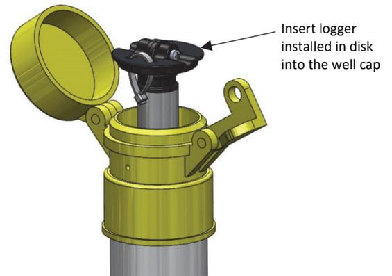
4. Close the well cap. Use the zip tie as a handle to pull out the logger and disk as needed.
