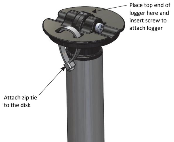
3. Place the disk with the installed logger into the well cap.
