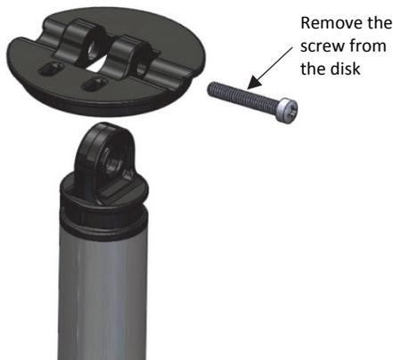
2. Insert the top end of the logger into the opening between the two raised holes on the disk. Slide the screw through all three holes and tighten it with a screwdriver. Attach the zip tie to the disk by feeding it through the two side holes as shown below.
