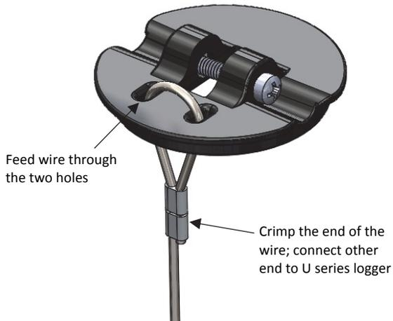
3. Insert the logger and disk into the well cap as shown in the example in step 3 of the MX2001 logger instructions.
