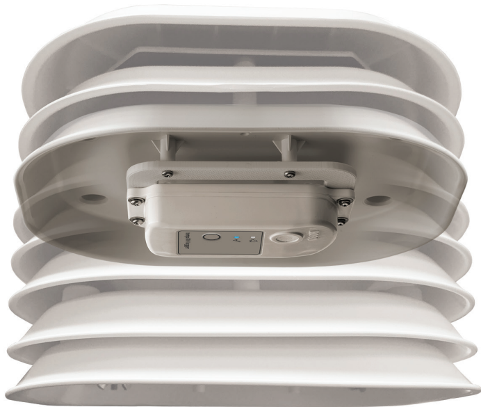
The HOBO MX2301 Temperature/Relative Humidity data logger shown mounted inside the RS1 Solar Radiation Shield
